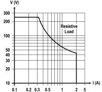
0.1 0.2 0.3 0.5 1 2 5 Mechanical / Electrical life:  $30 \times 10^6 / 1 \times 10^5$  operation, typical.
