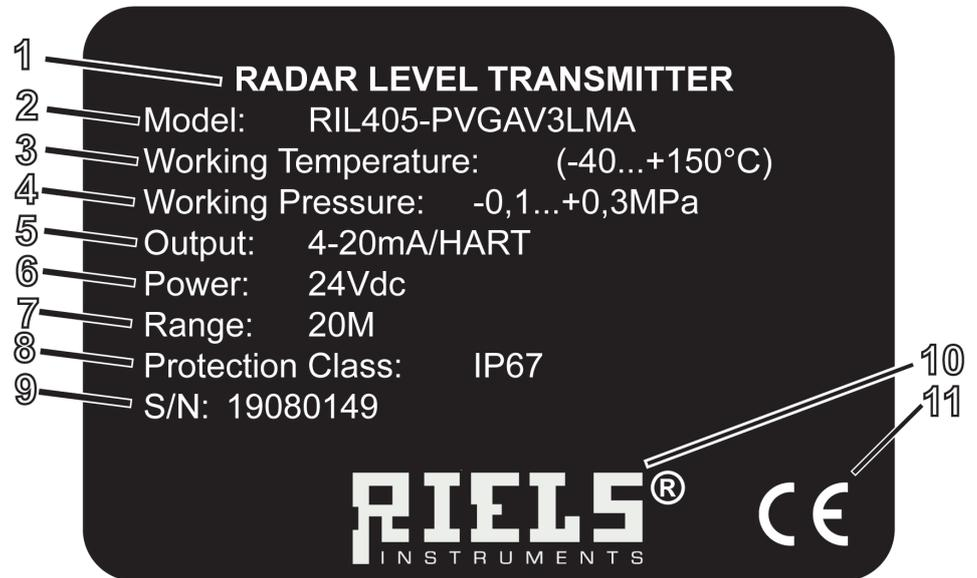
Fig. 1: Layout of the type label (example)
