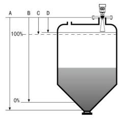
**Datum measurement:** Screw thread bottom or the sealing surface of the flange. **Note:** Make sure the radar level meter the highest level cannot enter the measuring blind area (Figure D shown below).
