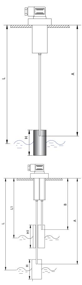
$\begin{array}{l} \textbf{L-LI} = 100 \text{ mm} \\ \textbf{A-B} = 90 \text{ mm} \\ \textbf{H} = 35 (L = 90 \text{ mm}) \\ \textbf{H} = 45 (L = 100 \text{ mm}) \\ \textbf{H} = 55 (L = 110 \text{ mm}) \\ \textbf{H} = 60 (L = 120 - 500 \text{ mm}) \\ \textbf{H} = 90 (L = 501 - 1000 \text{ mm}) \\ \textbf{H} = 35 (LI = 90) \\ \textbf{H} = 45 (LI = 100) \\ \textbf{H} = 70 (LI = 120 - 1000 \text{ mm}) \end{array}$
