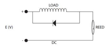
When the circuit is alternating, the diode cannot be used. Therefore an arc suppression unit must be used; in general this is a block of resistances and capacitances connected together in series and in parallel with the reed.
