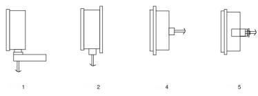
I Wall with bracket; bottom output. 2 Wall with 3 holes flange; bottom output 4 Panel with 3 holes flange; back output 5 Panel with U clamp; back output
