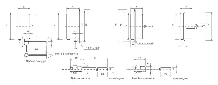
The 'S' dimension must be determined so that the sensitive part of the bulb is completely immersed in the process fluid.
