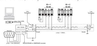
Line termination must be set at the two network ends. To polarize the line during nontransmission periods, resistor are connected between signal and power supply lines. The maximum number of devices that can be connected to the (Bus) line RS485 depends on the load characteristics of the devices to be connected.
