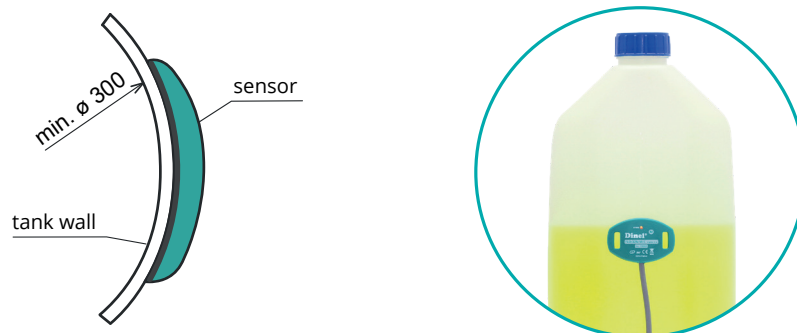
Fastening the FLD-32 using self-adhesive layer
