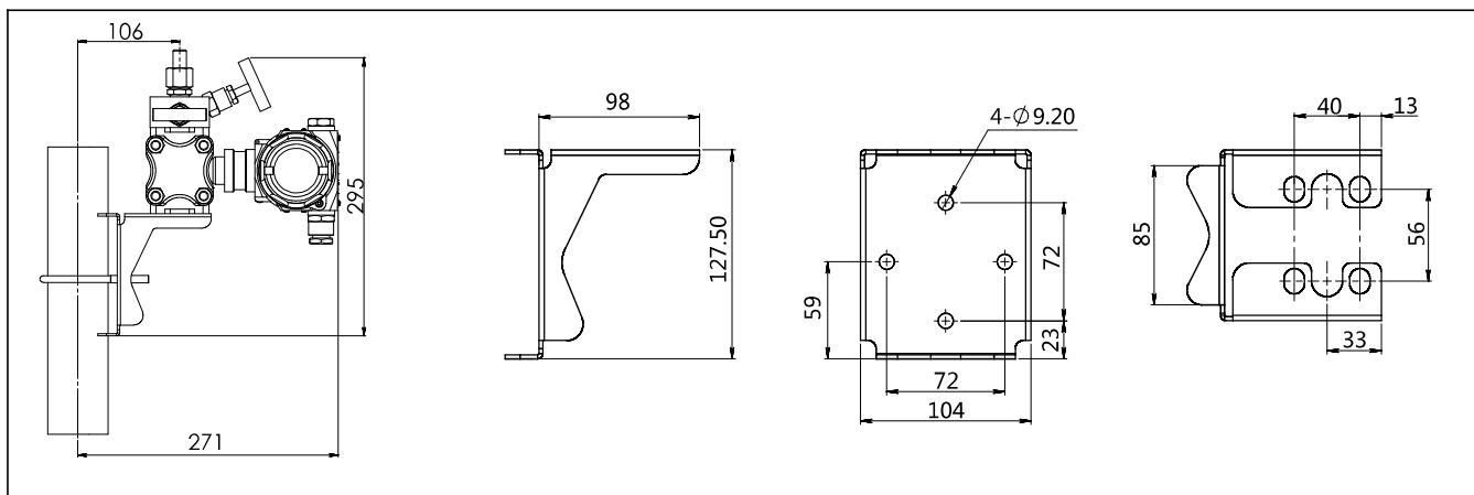
Plate mounting bent bracket(B2) drawing and dimension (unit:mm)
