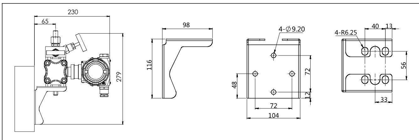
Pipe mounting flat bracket (B3) drawing and dimension (unit:mm)
